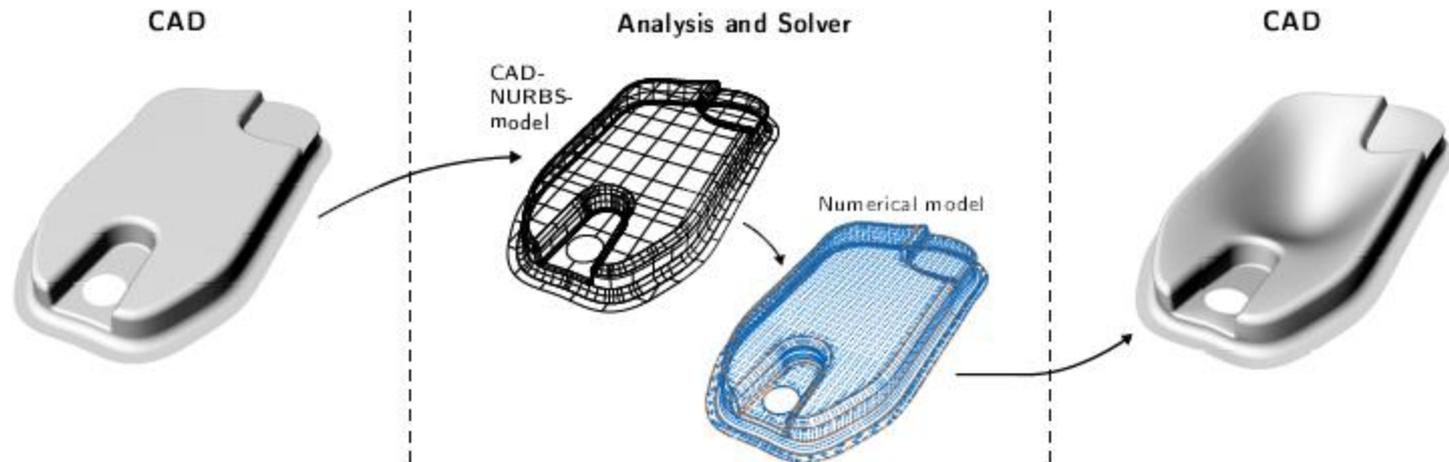
Realization of CAD-integrated Shell Simulation
