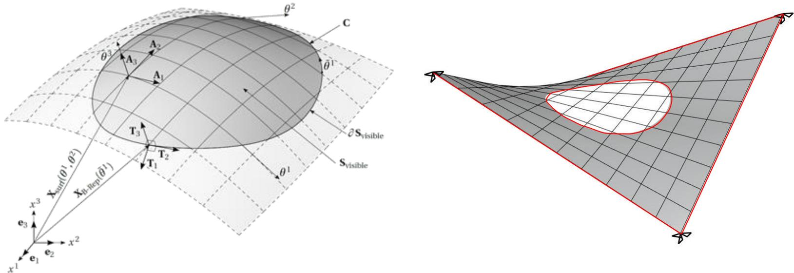
For membrane theory to be applied, we are adding extra stiffness on the boundaries (cables)
